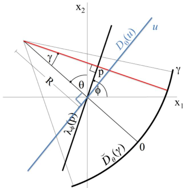
The blue line represents the straight detector, virtually positioned at the isocenter (origin)
