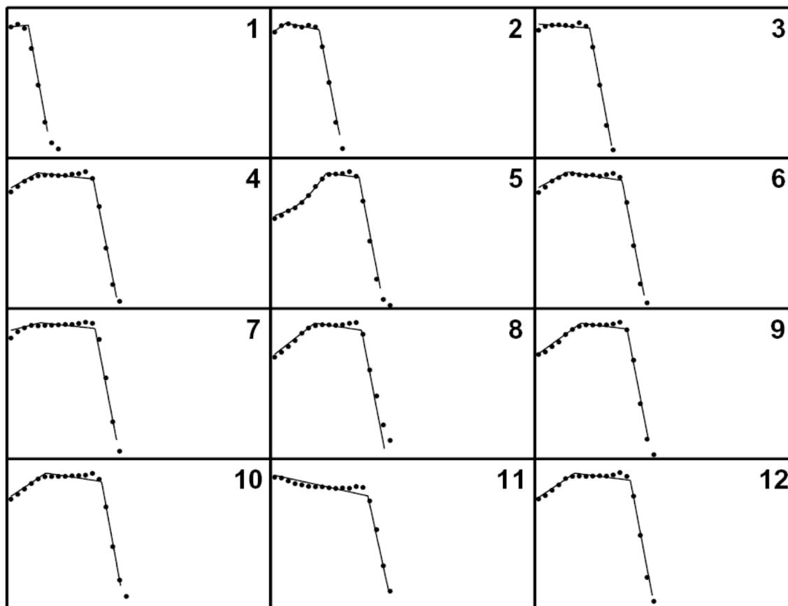
Further comparisons with diode scans. Dots = diode wheel, line = fit to MLIC scan. As did the previous slide, most of these show the slight peakiness expected from the diode's higher response at low energy. That could be handled by looking for a slightly non-flat MLIC result, but problems measuring the output factor for very small fields have so far kept the MLIC from use in patient eye calibrations. It is used for daily QA.
