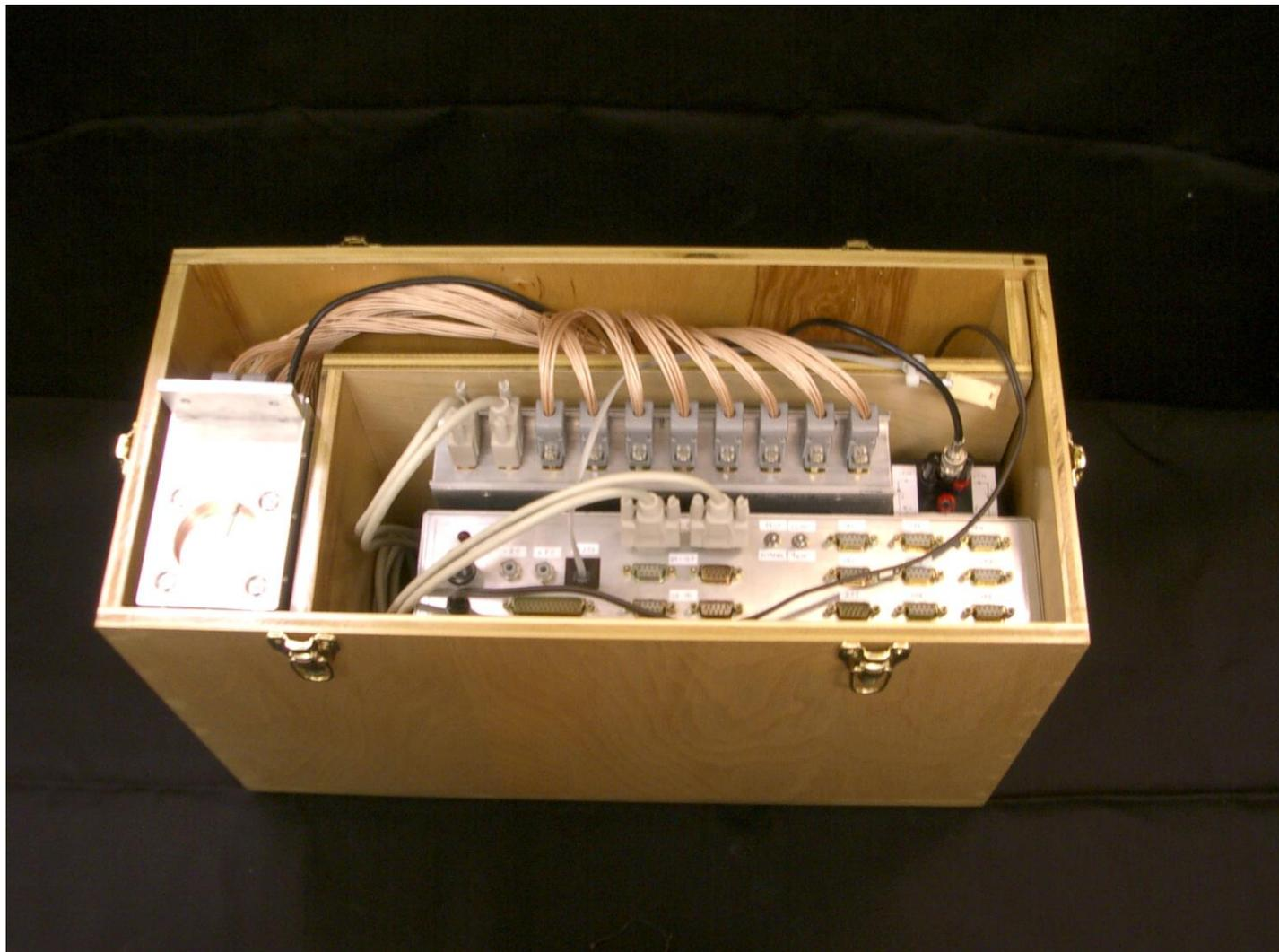
Treatment rooms are hostile environments for equipment so thought should be given to storage and ease of setup. The MLIC is kept in a case along with its electronics. Battery-supplied HV is on permanently (BNC cable) for stability of operation. The box is carried to the beam line, the MLIC is removed and mounted, and the power cord and RS-232 modular phone line are plugged in.
