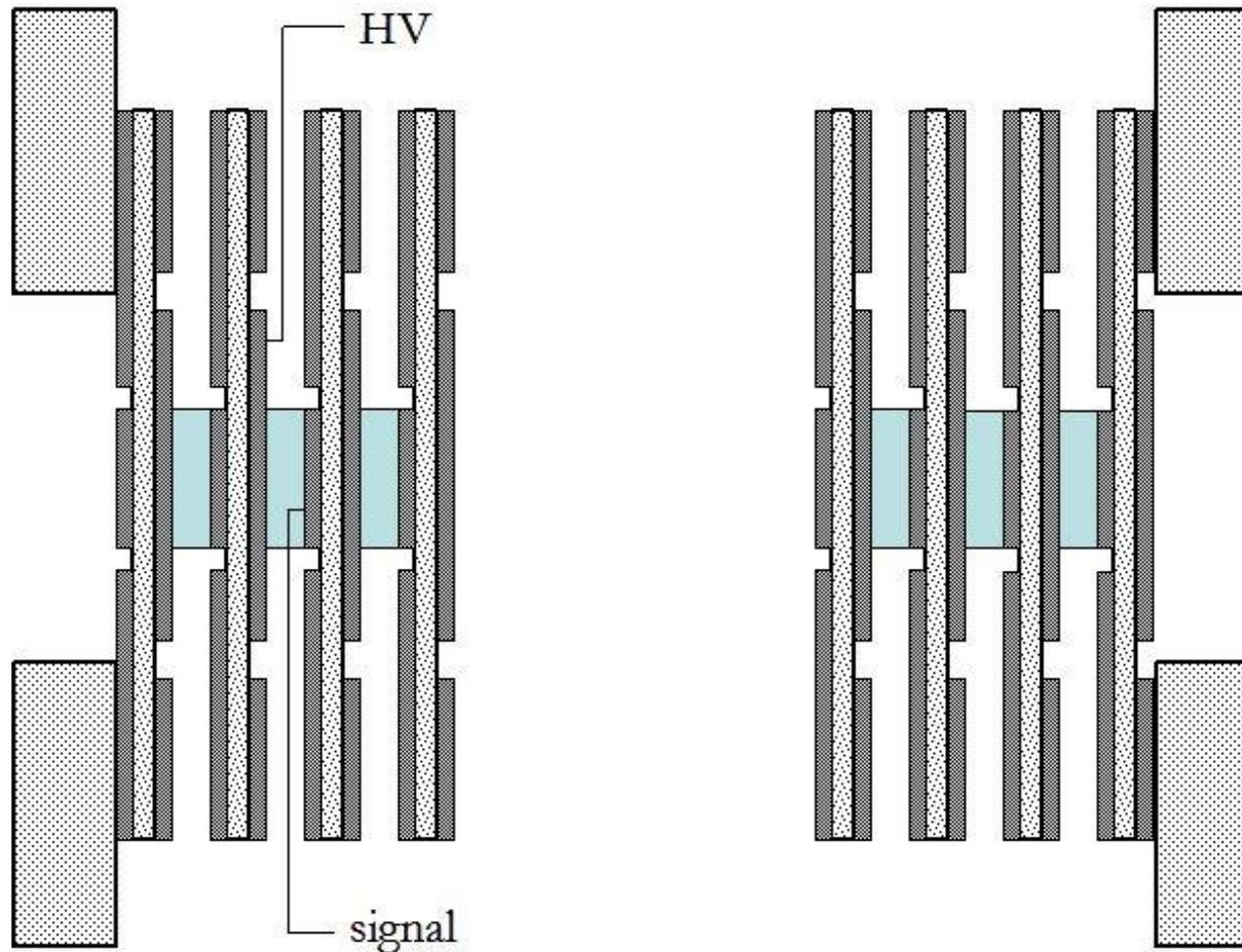
(*Not to scale.*) Identical PC boards with a signal pad on one side, and a (larger) HV pad on the other, form an array of small PPIC's. Grounded guard surfaces make the field uniform in the region of interest. The board and copper provide energy loss, the gap provides active volume, and the whole is proportioned to be roughly water equivalent.
