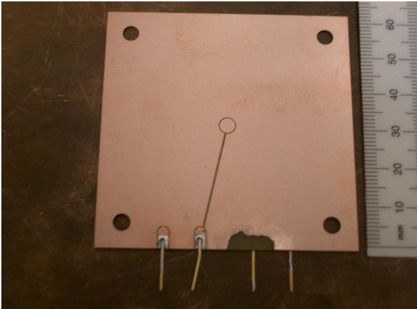
The 4 mm diameter signal pad is surrounded by ground plane. The gap between them is as small (0.006") as can be manufactured reliably, to reduce the number of protons that lose slightly less energy because they go through the gap. Signal and ground are brought out to square pins soldered by hand (note the thermal relief). Copper was removed by hand to avoid having 100 V across the 0.020" board edge.
