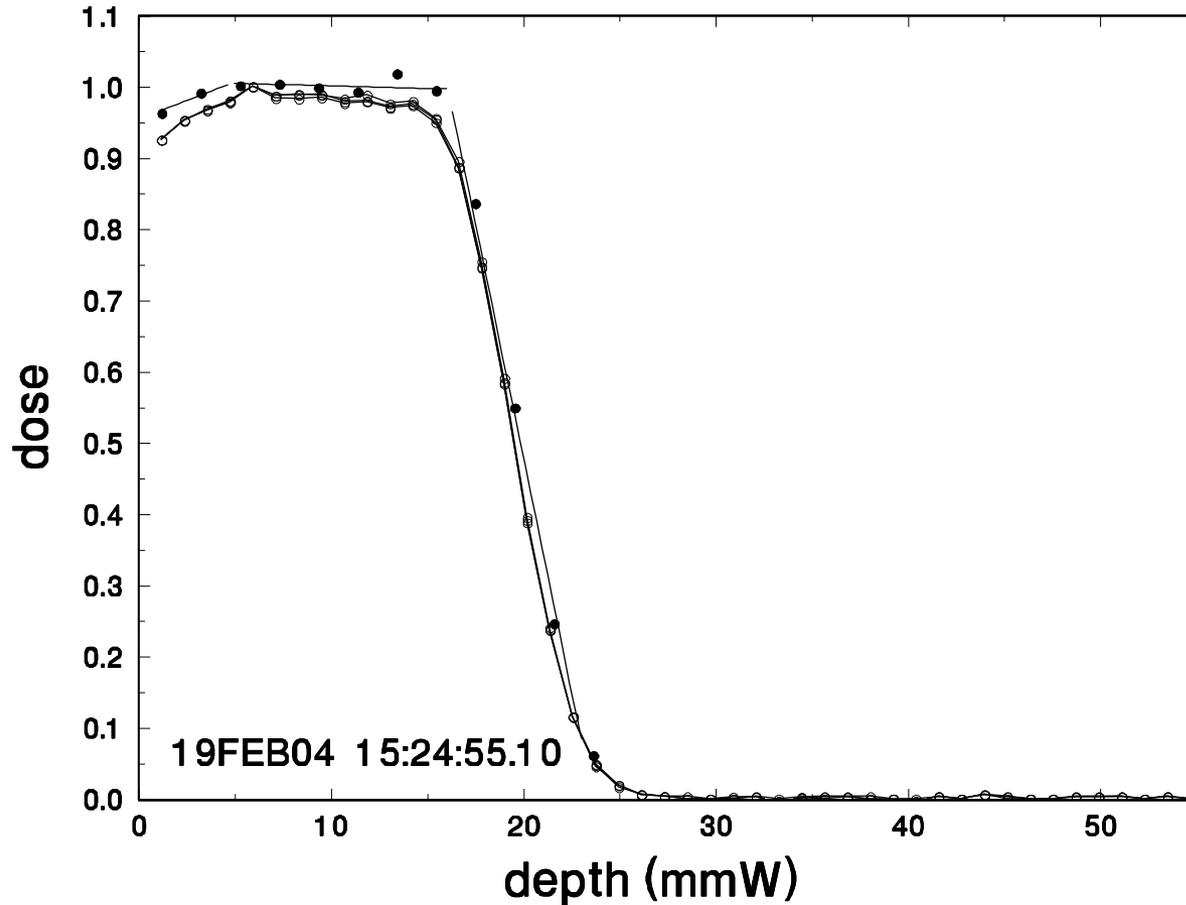
MLIC measurements on a number of patient eye fields were compared with diode scans using the traditional AMK/diode wheel method, the gold standard at the Burr Center. This is a typical comparison: filled circles = diode scan (about 8 minutes if you get to keep the beam), open circles = several MLIC runs (2 seconds each).
