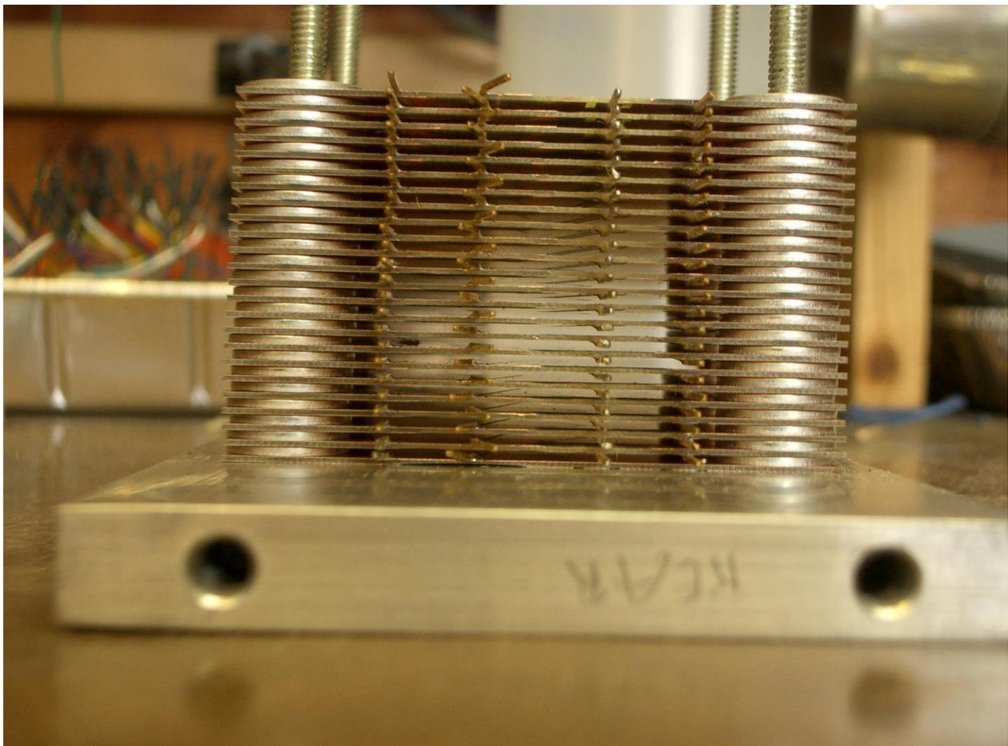
The boards are separated by ordinary flat washers. The square pins just miss the opposing board. Capturing the board with the threaded rods was not a good idea, as it is tedious to fix assembly errors and possible future faults. The assembled stack by itself tends to twist as the screws are tightened. It totally relies on the frame to keep it square!
