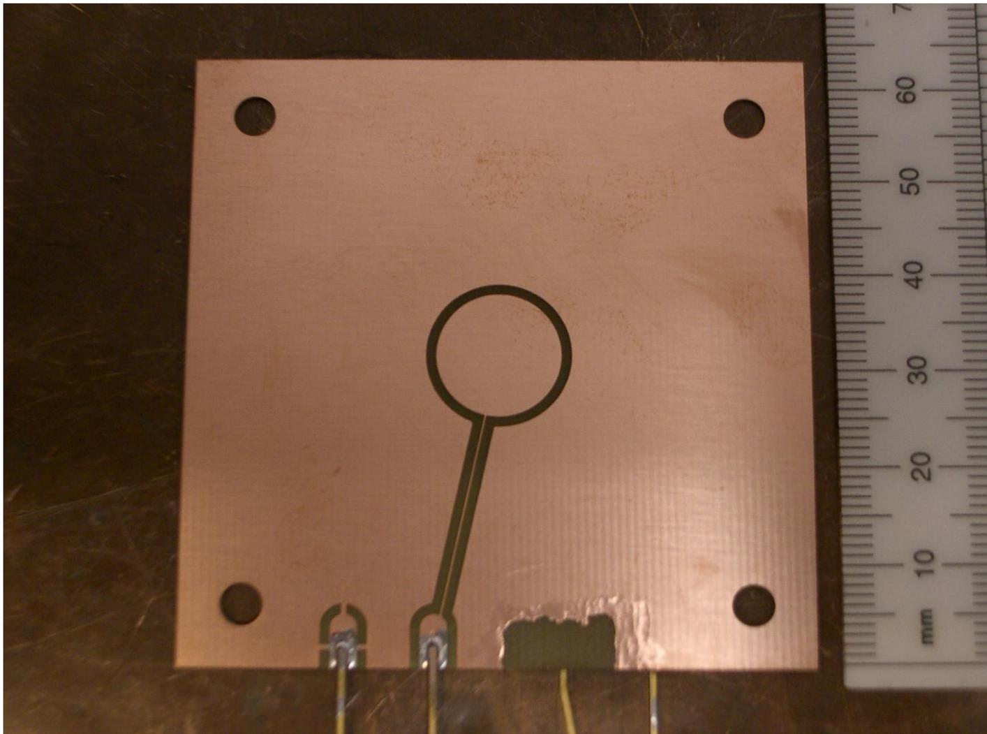
The 0.5" HV pad is also surrounded by ground plane. The copper-free space is larger to accommodate the HV and because it does not matter: protons this far out will never make it to a signal pad. The HV pad, with the ground plane facing it, provides a uniform field over the active volume. The field further out is non-uniform but doesn't matter. The limited HV pad area reduces superfluous current when the beam is on.
