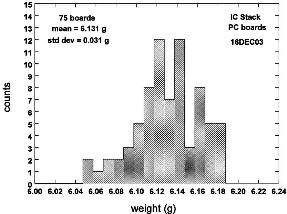
Before preparation for assembly the boards, whose area is essentially identical because of the fabrication process, were weighed. The mean weight was 6.131 g with an rms spread of  $\pm 0.031$  g (0.5%). The outliers were set aside and the rest treated as equal. A  $\pm 0.5\%$  difference in the width of individual channels (differential nonlinearity) is insignificant in a depth-dose measurement.
