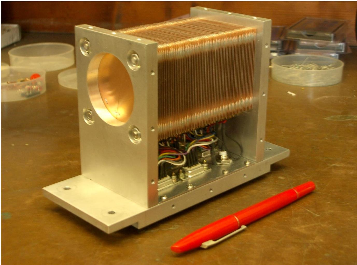
65 identical PC boards, fabricated with standard commercial technology, are mounted 1 mm apart in a rigid frame. Collimation is provided by the eye treatment line. The defining aperture or natural beam size must be much smaller than the hole shown. Otherwise, the connections are bathed in ionized air and contribute garbage signal.
