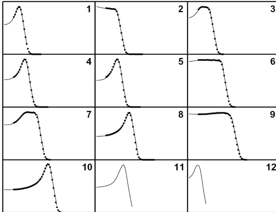
Later, MLIC measurements were compared to identical pristine and SOBP's measured in a water tank using a Markus PPIC (data courtesy Wayne Newhauser and Nick Koch). The graph shows the water tank data (dots) compared to a *fit* to the MLIC data (line). In many cases it almost seems that the water tank data are being fit!
