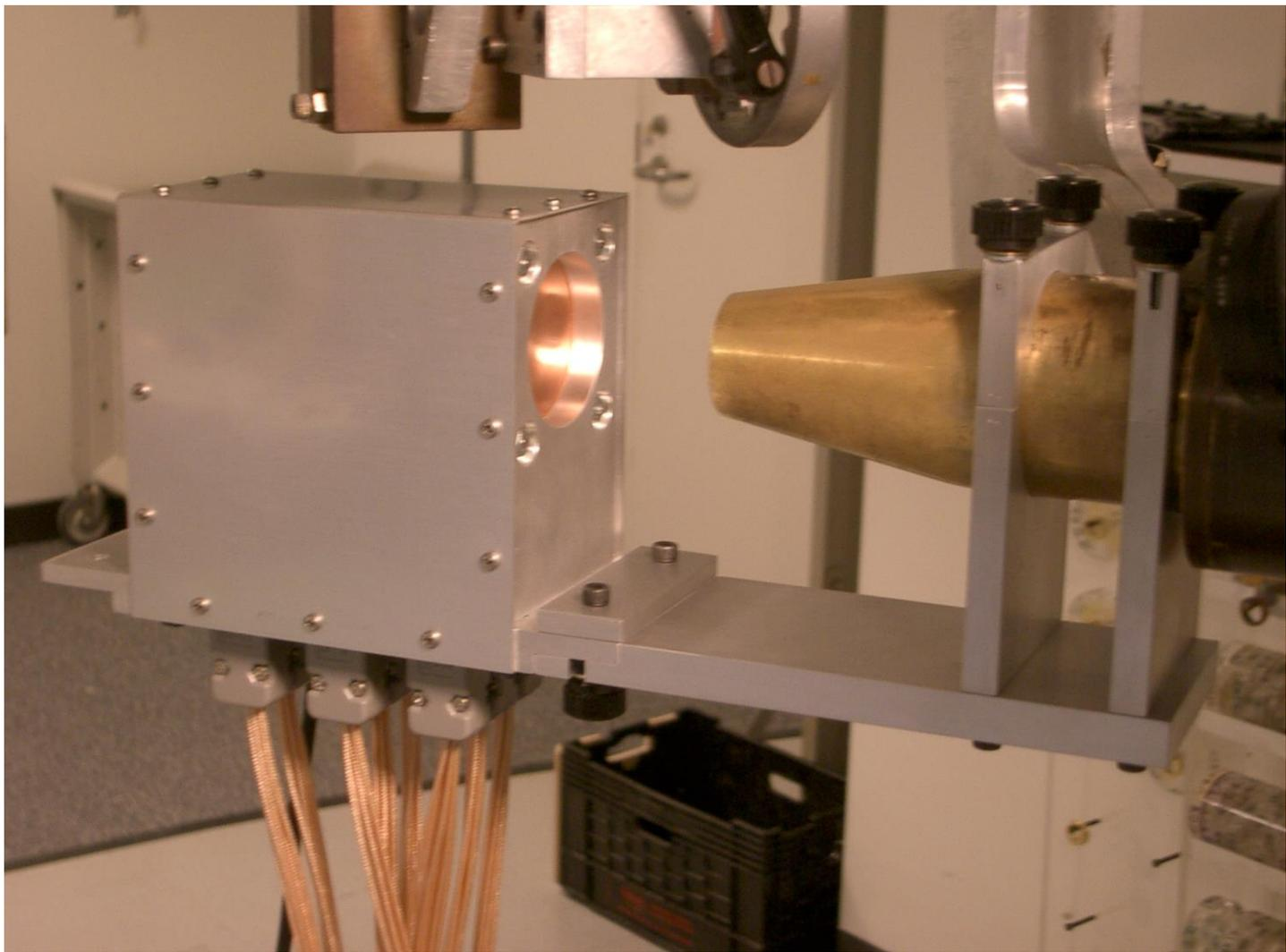
It takes longer to set up an array device than to take the measurement, so the mechanics should be carefully thought through. The 'eye MLIC' is mechanically compatible with the diode scan device used traditionally. A field light projected onto the (unused) front signal pad facilitates alignment, and sideways motion accommodates eccentric apertures. The MLIC and frame are end-to-end symmetric to pass a high energy beam either way.
