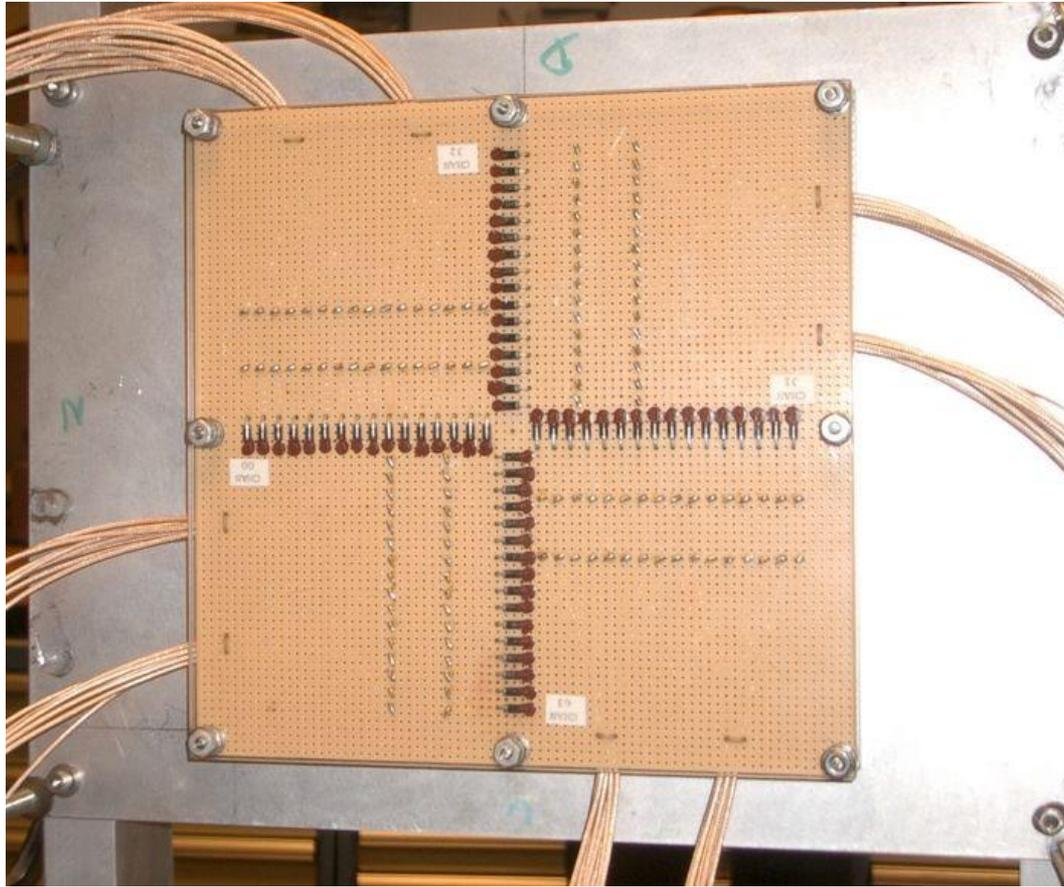
The  $32 \times 32$  'CROSS' diode array built for QA in the HCL radiosurgery beam and now used for general purposes at the Burr Center. 1N4004 diodes are mounted on perfboard at 0.2" pitch. Leads not at ground are covered with insulating paint to discourage ion collection. The diodes put out so much signal (130 pC/rad) that they will not reach the 10 Krad damage threshold in the lifetime of the device, so they are *not* pre-irradiated.
