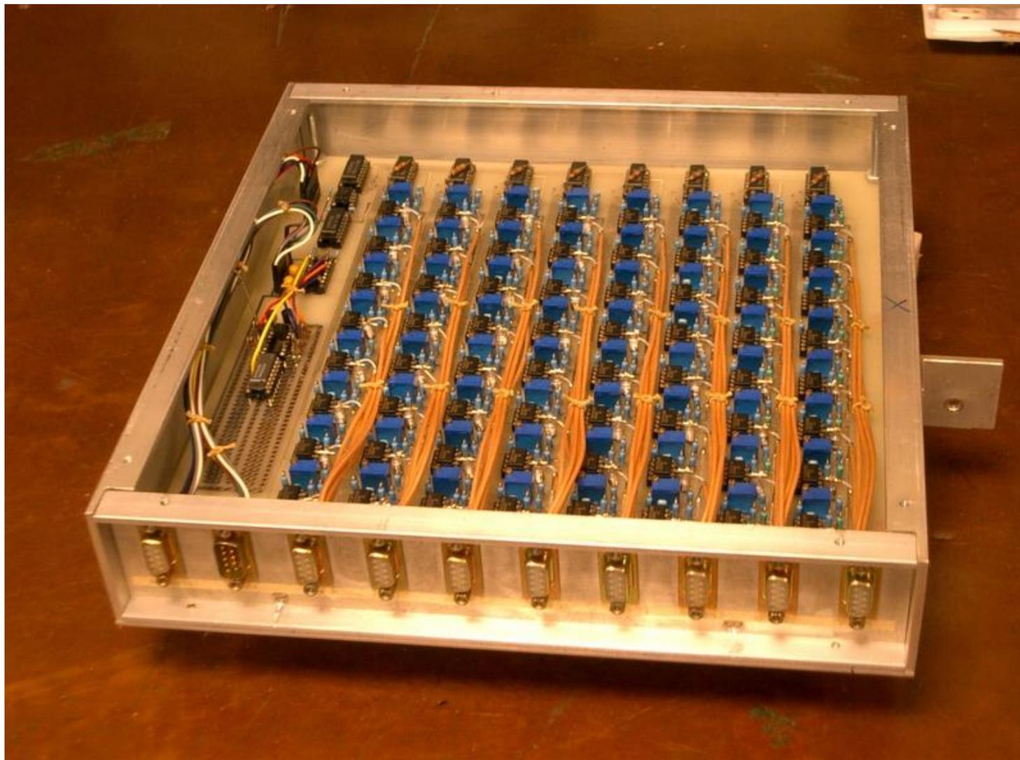
This array is used at the Burr Center for CROSS and MLIC. A second unit houses a scanning ADC to read the integrators and transmit data to a host computer via RS-232.
