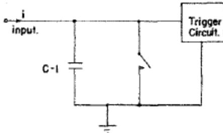
FIG. 2. Modified integrator circuit.
