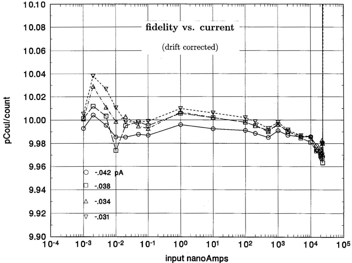
$\Delta Q$  is independent of input current over >7 decades to  $\pm 0.2\%$ . Even during a hypothetical high-current accident this circuit will keep track of the dose delivered.
