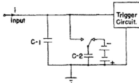
*Classical* integrator. When the voltage across  $C_1$  reaches some level, discharge  $C_1$  by closing the switch. During this time, current is lost. Accuracy depends on the stability of  $C_1$  (no problem) and the stability of the threshold level. Residual charge at the end of measurement may be significant.
