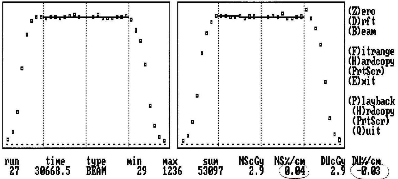
On-line displays on the PC running the CROSS array. The measurement shown took *two seconds*. Array devices take longer to set up than to use so ease of setup should guide the mechanical design. Data should be recorded in a compact and automatically named *log file* with no operator response needed.
