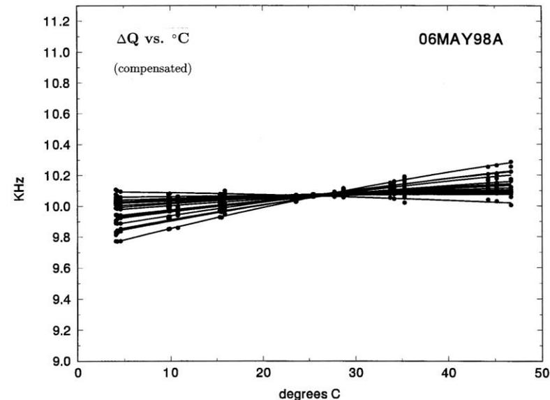
Analog circuits always have temperature dependence, which is tricky to measure because the board must be heated or cooled *uniformly*. Without compensation, the recycling integrator has a temperature coefficient (‘tempco’) of  $\approx -0.25\%/^{\circ}\text{C}$ . It can be compensated by varying ‘+5 V’ very slightly. That adjusts  $\Delta Q$  without significantly affecting circuit operation.
