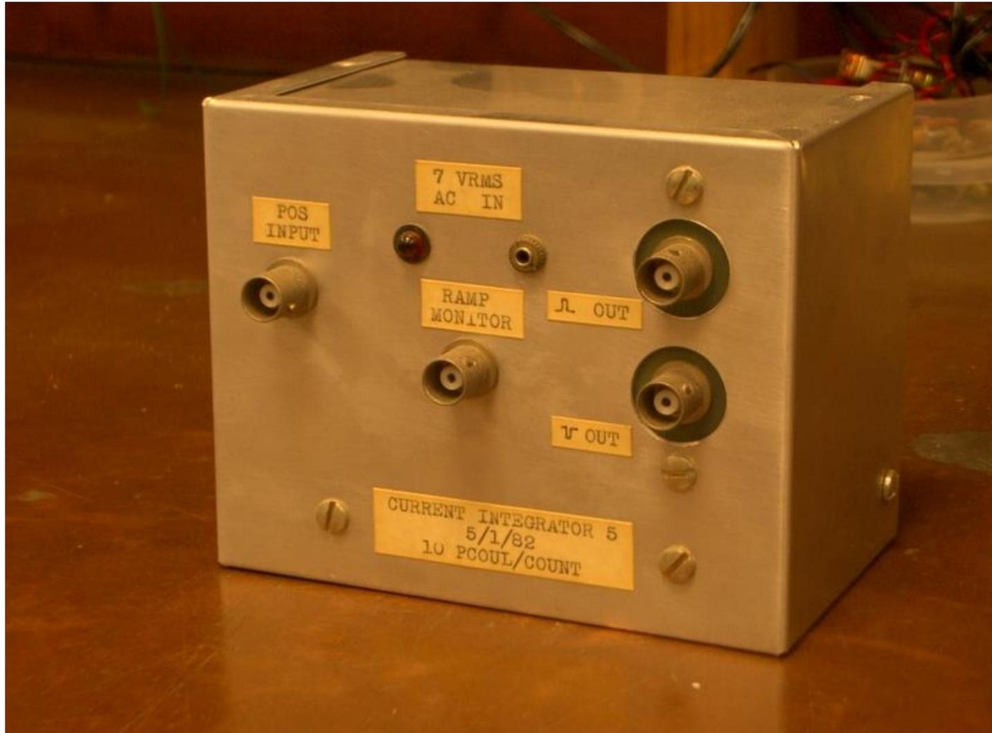
Single channel line powered recycling integrator used with beam monitor IC's at HCL and for general purposes at the Burr Center. Sinks charge, puts out a pulse for every 10 pC.
