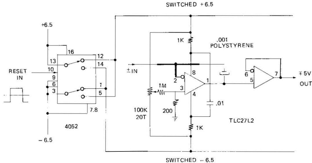
From B. Gottschalk, 'Resetting a current integrator with the supply lines,' Nucl. Instr. Meth. **A297** (1990) 534. Instead of using a relay or transistor, this integrator is reset by reversing the supply lines through current limiting resistors. That effectively puts the capacitor inside a conducting diode bridge. This circuit has a very low parts count which, along with the 'memory' provided by the integrating capacitor, makes it ideal for arrays read out by a single scanning ADC.
