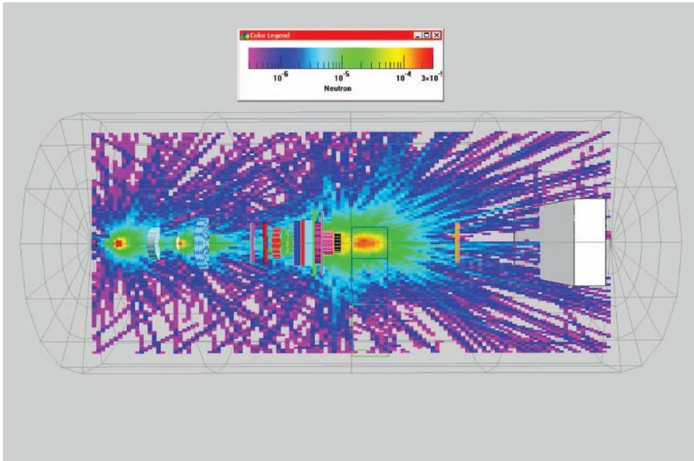
Moyers et al., 'Leakage and scatter radiation from a double scattering based proton beamline,' Med. Phys. **35** (2008) 128-144 : fluence for neutrons  $>10$  MeV. Neutrons reaching the patient (green) are mainly from collimators near the patient. Stop protons as far upstream as possible!
