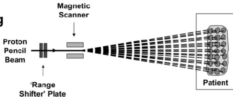
Fig. 9. The protons emerging from a cyclotron or synchrotron form a narrow pencil beam. To cover a treatment field of practical size, the pencil beam must be either scattered by a foil or scanned. Passive scattering is by far the simplest technique but suffers the disadvantage of increased total-body effective dose to the patient.
