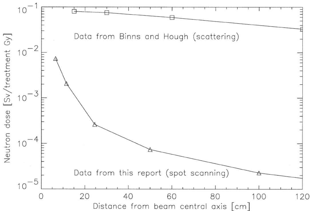
Schneider et al. Figure 3. The external dose is broader than the internal dose because the external source is upstream of the patient. (Think of a garden hose set to spray.) Organs *transverse* to the target may receive nearly all their dose from external neutrons!
