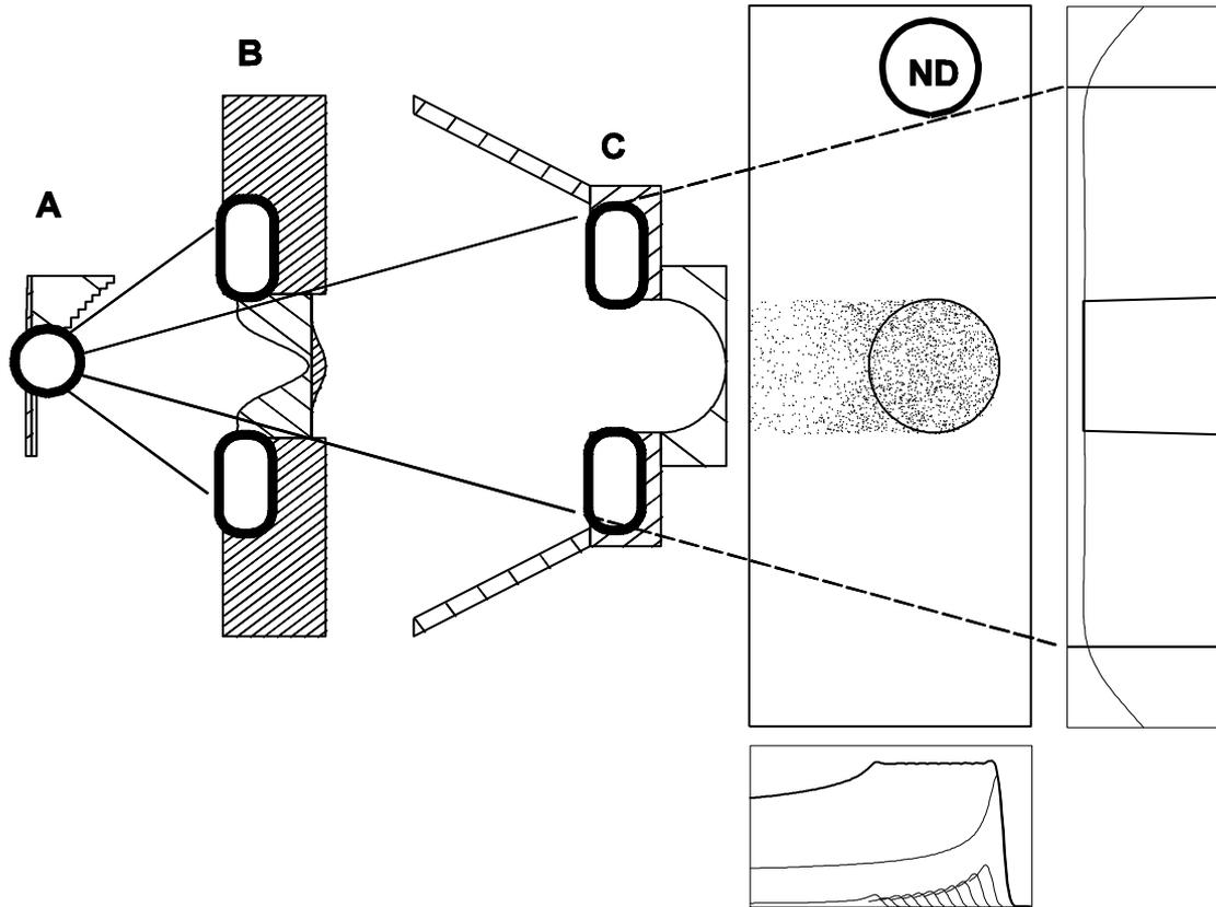
Neutrons arise wherever *many protons* lose *a lot of energy* : the range shifter/modulator, the collimator around the second scatterer B and the patient aperture C.
